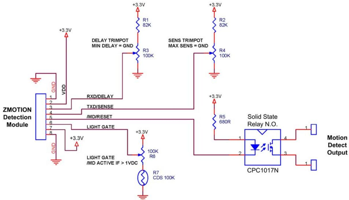
Figure 11. Application Example - Hardware Interface Mode
