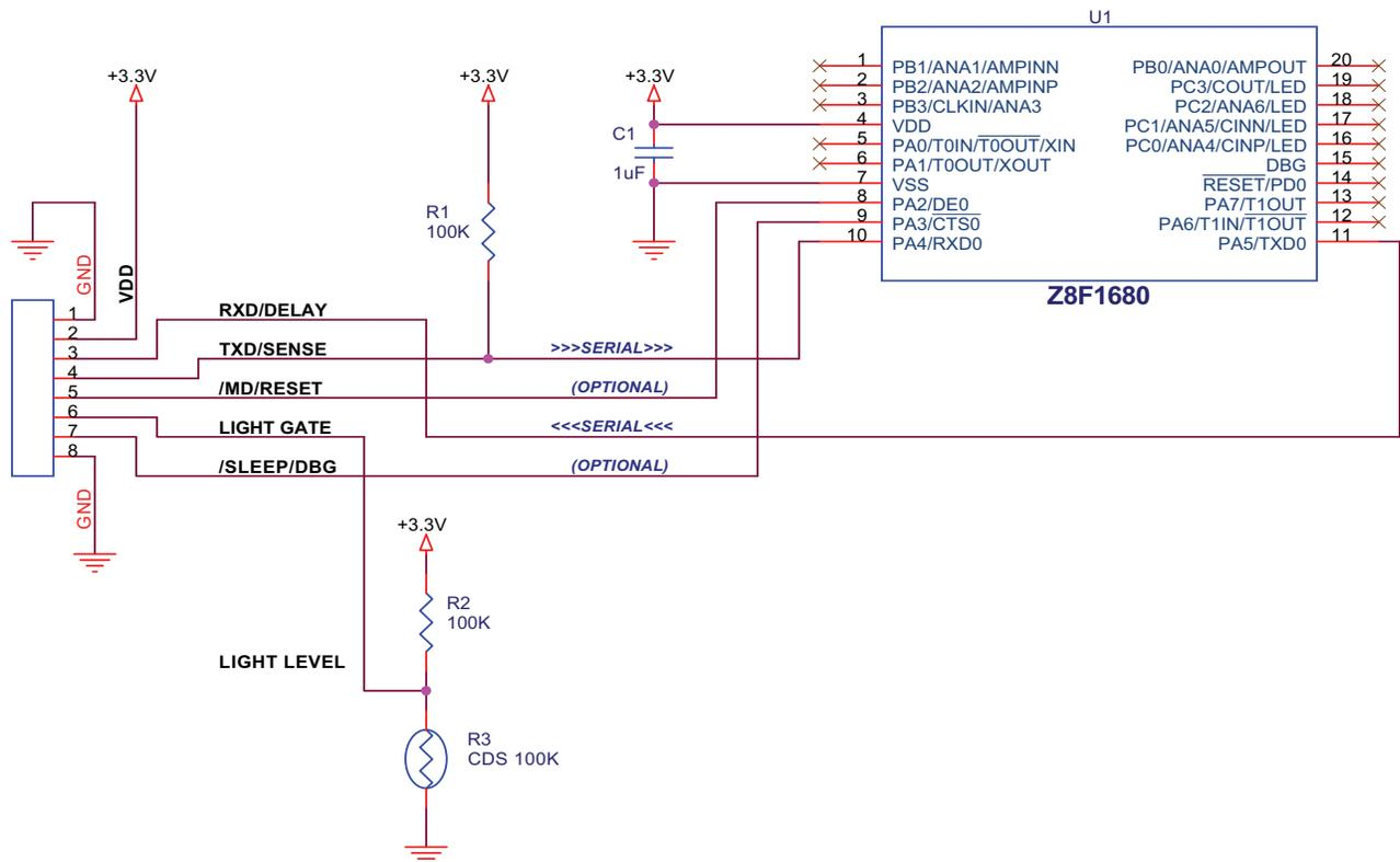
Figure 12. Application Example - Serial Interface Mode
