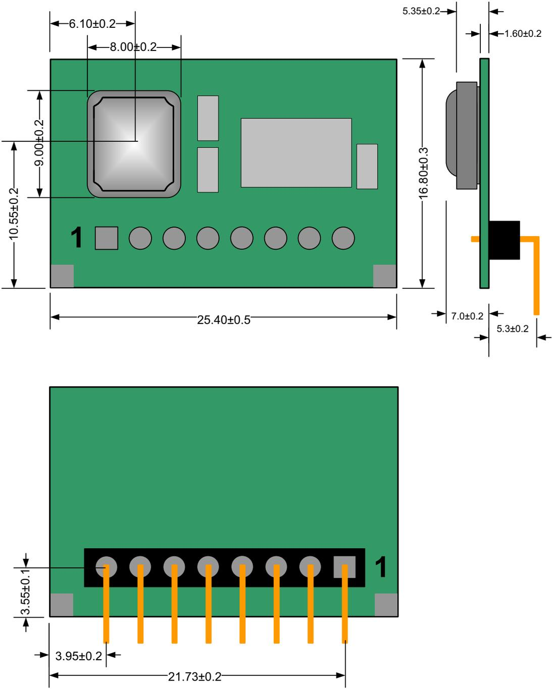
**Figure 9. Mechanical Drawing of ZMOTION™ Detection Module**
