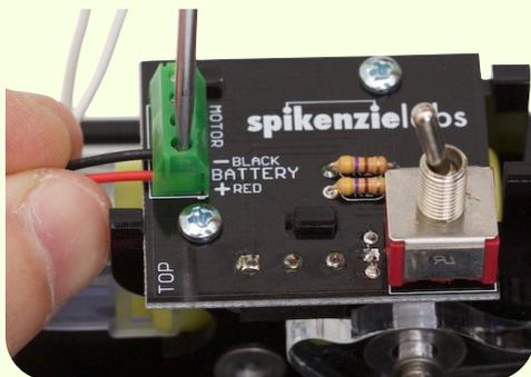
**Note:** Make sure to tighten the screw terminals onto the bare wire, and not the colored plastic casing. You may have to loosen the screw terminal in order to get the wire in.
