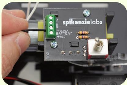
The red wire from the battery pack goes to the **+RED** screw terminal. Screw both in place.
