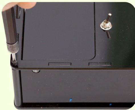
Only screw the top screws in until they touch the top piece of acrylic. If the corner posts are not flush, the top will flex. It is ideal to have the top piece laying flat.
