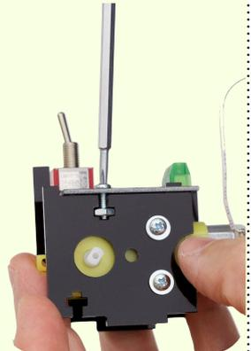
In the same way, slide in the other nut, on the other side, and attach the other screw.
