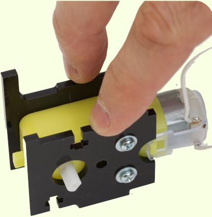
With the screws a little loose, press down against a flat surface, so that the both bottoms of the motor mount are flat.
