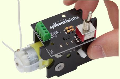
You will be using these nuts and screws to hold secure the PCB to the motor mount.
