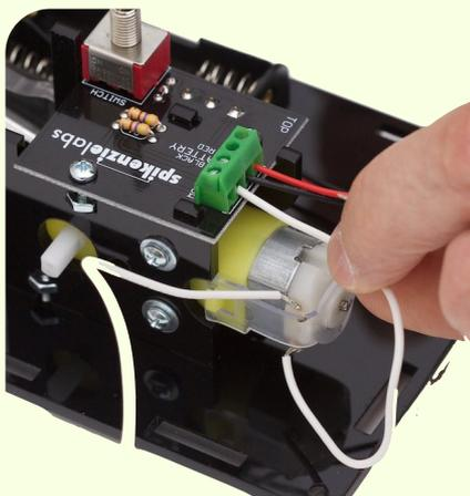
The top wire from the motor connects to the last screw terminal. Slide it in place, and screw it down.
