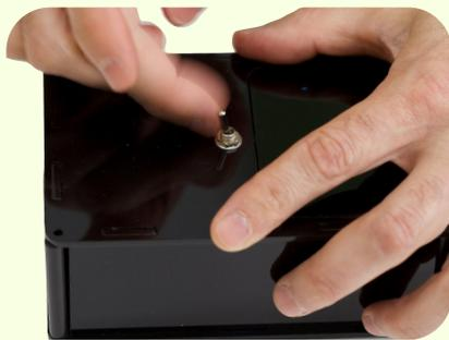
The remaining 4 black screws get sent through the holes in the corners of the top cover. Make sure that the screw and the round corner pieces are lining up as you go. Once again, do not over-tighten.
