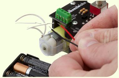
Touch the red and black wires to the wires connected to the motor. Pull one of the wires away and check the position of the motor shaft. Repeat until you have the motor shaft at a 12 o'clock position. Really close is good too. Once done, remove the batteries from the holder and set it aside.
