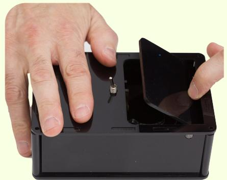
Once the top panel is set, take the washer, and place it over the toggle button. (Curved side up)
