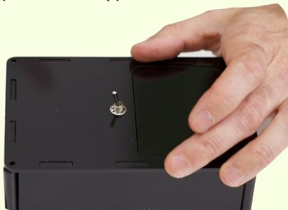
Screw the nut down, finger tight only. Do not use any tools for this.
