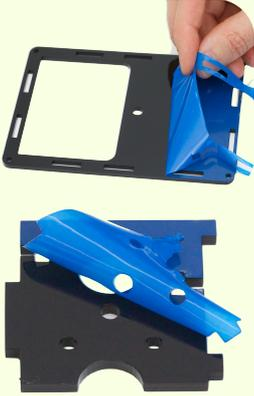
Etched parts are covered by a special masking tape. Sometimes the glue from the tape is difficult to remove. If there is stubborn glue residue left from the masking tape, the best way to clean it is using some WD-40, which will remove the glue.
