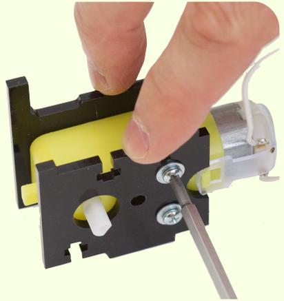
Keeping the bottoms of the motor mount flat against the surface, tighten both screws.
