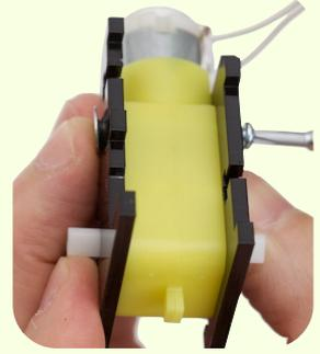
While holding the weld nuts in place, slide both screws through the washers, motor mount, motor and screw into the weld nut. For the moment, leave the screws loose enough so that the motor mount plastic can wiggle a little.
