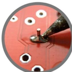
Allow solder to flow onto pin and pad.
