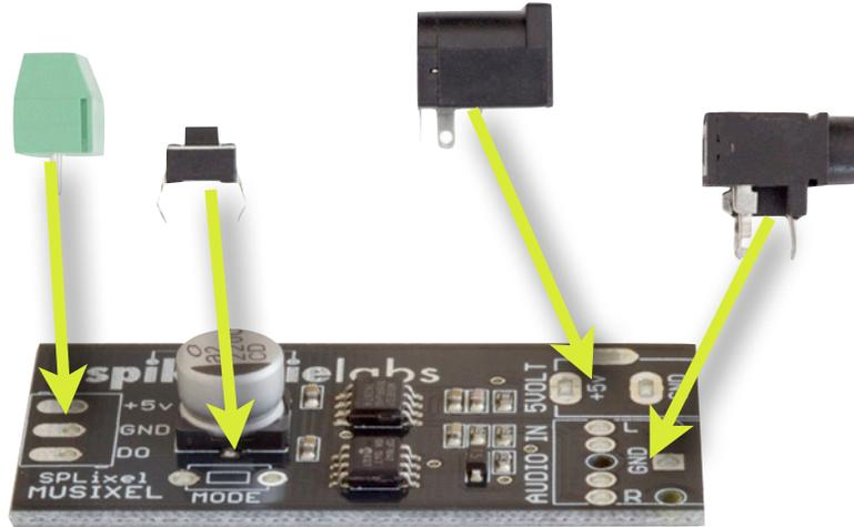
Place the parts onto the PCB. Make sure the openings point towards the outside of the board.
