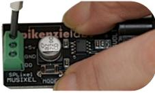
Loosen the screw terminals a little to allow the wires to slide in. ~ 3 turns
