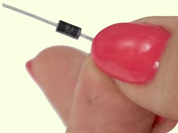
Grasp the diode a little bit away from the body, and bend the legs similar to the way you prepared the resistors.
