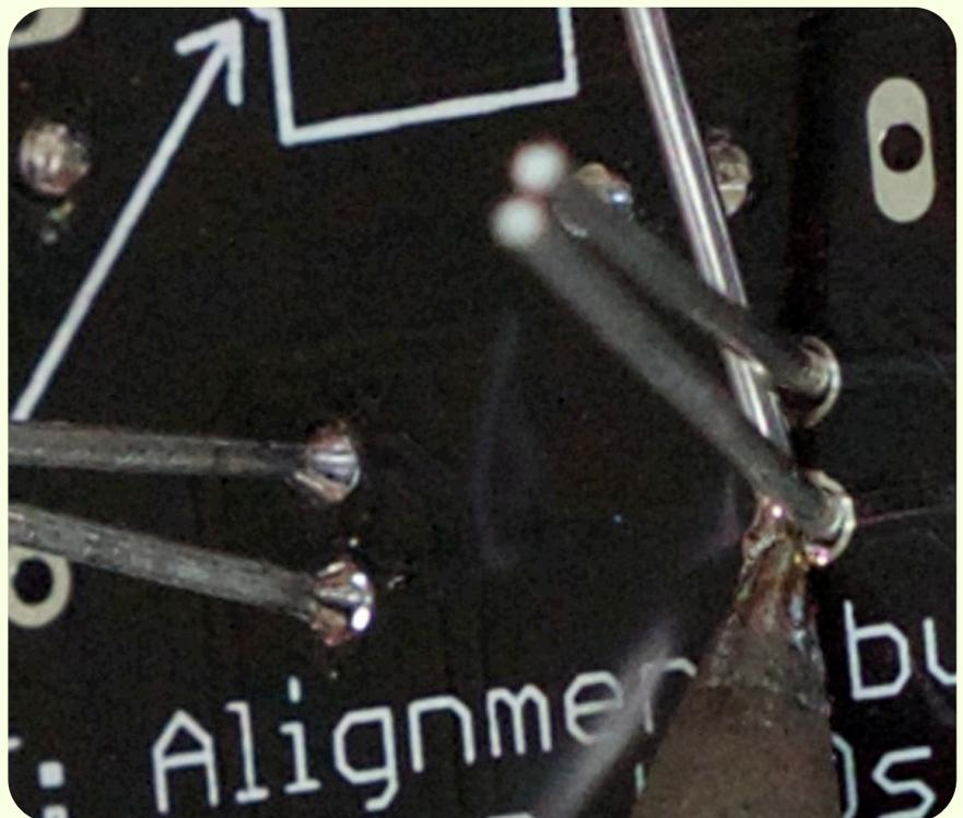
Once you have soldered and snipped these diodes into locations D1, D2, and D3, continue to the next step.
