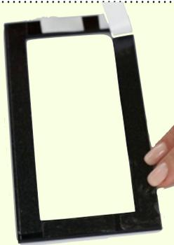
Remove the slippery white double-sided tape covering from one of the bezels
