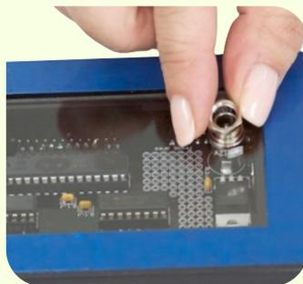
Take the remaining black screw, and finger tighten it through the hole into the rear structural layer.
