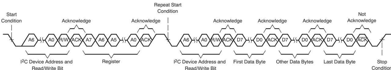
Figure 40. Multiple-Byte Read Transfer
