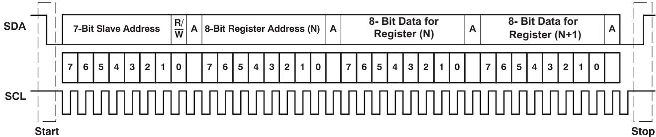
Figure 36. Typical I<sup>2</sup>C Sequence
