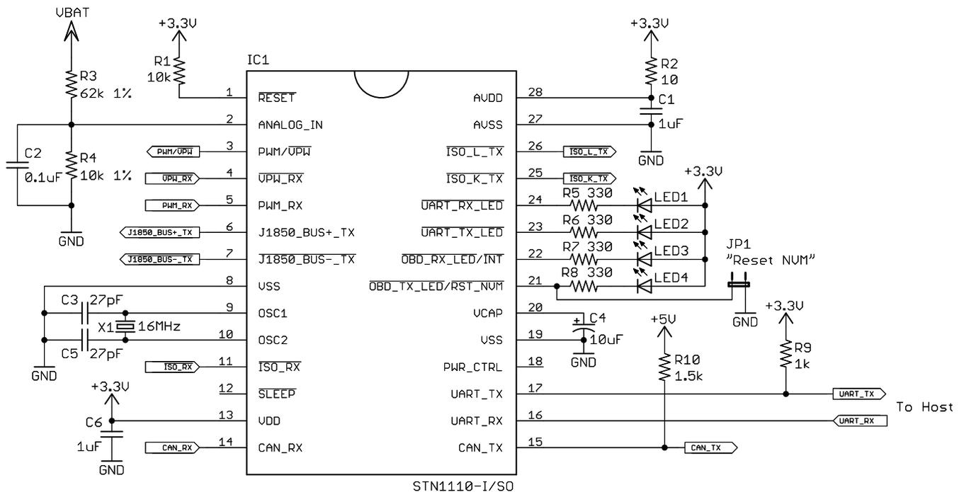
Figure 3 – OBD Connections
