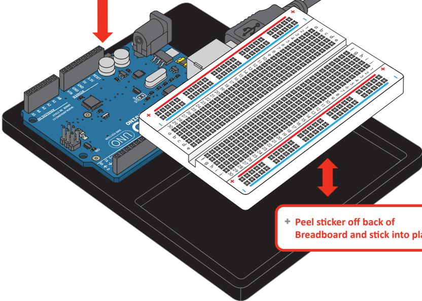
+ Peel sticker off back of Breadboard and stick into place.
