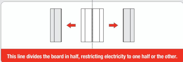
This line divides the board in half, restricting electricity to one half or the other.
