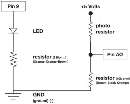
So you've already played with a potentiometer, which varies resistance based on the twisting of a knob. In this circuit, you'll be using a photo resistor, which changes resistance based on how much light the sensor receives. Since the Arduino can't directly interpret resistance (rather it reads voltage), we use a voltage divider to use our photo resistor. This voltage divider will output a high voltage when it is getting a lot of light and a low voltage when it is not.
