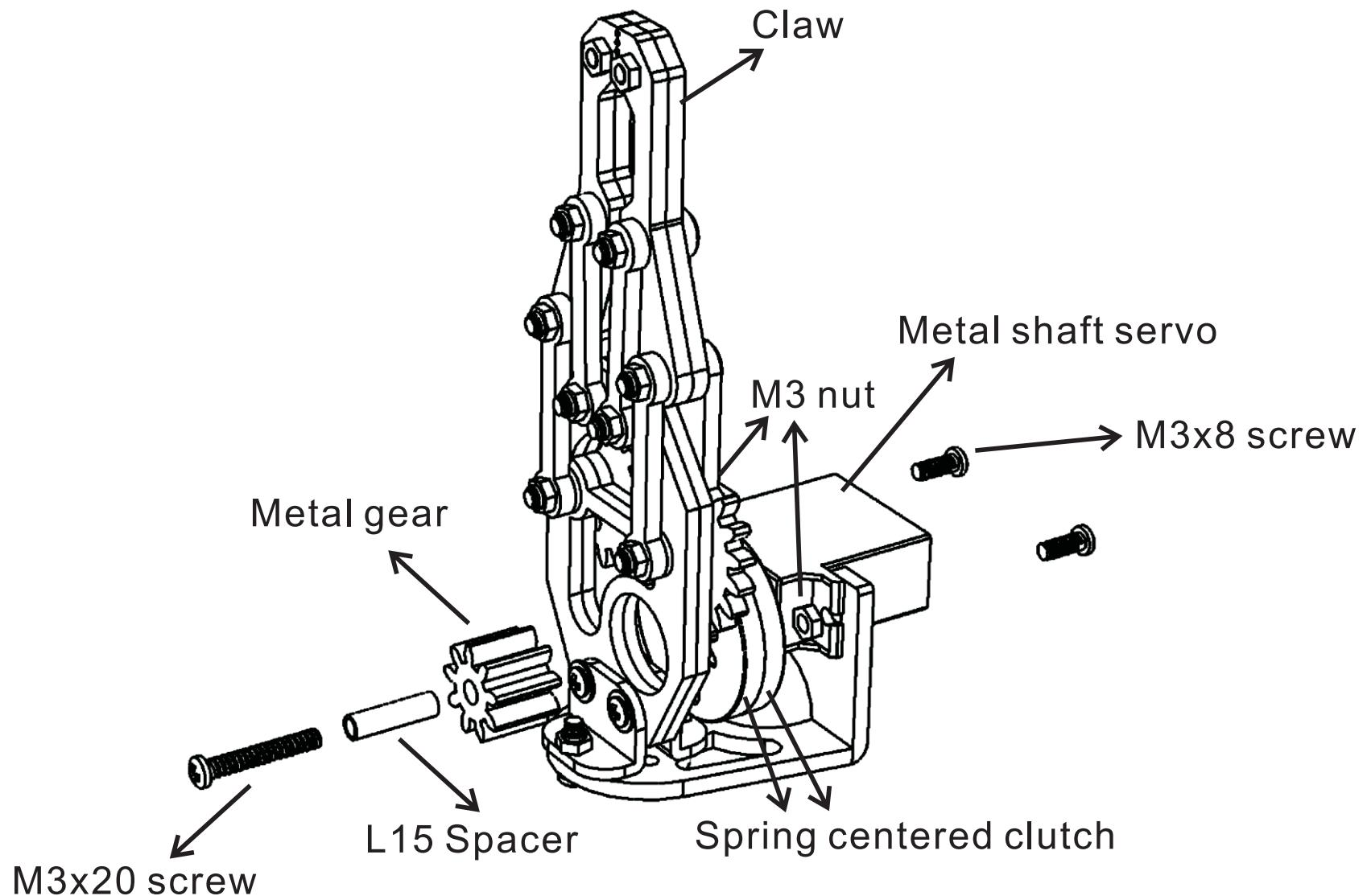
**It is suggested to make the servo shaft turn in the middle position when assembly the clutch.**
