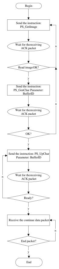
d) Reading a appointed template from flash fingerprint database and uploading;
