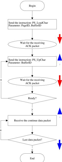
e) Reading an image from sensor and searching the database field from 10—100.
