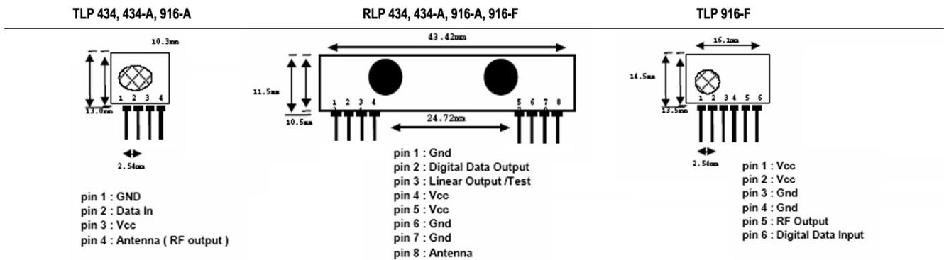
These devices are simple pass-through integrated circuits. Meaning, you set up your baud-rate (as long as its within an acceptable range of whatever pair of devices you are using), and then start sending bytes to the transmitter. Quite simply, it just sends your data out the transmitter and the receiver grabs it, acting as if you had a wired serial connection between them, minus the wire!
