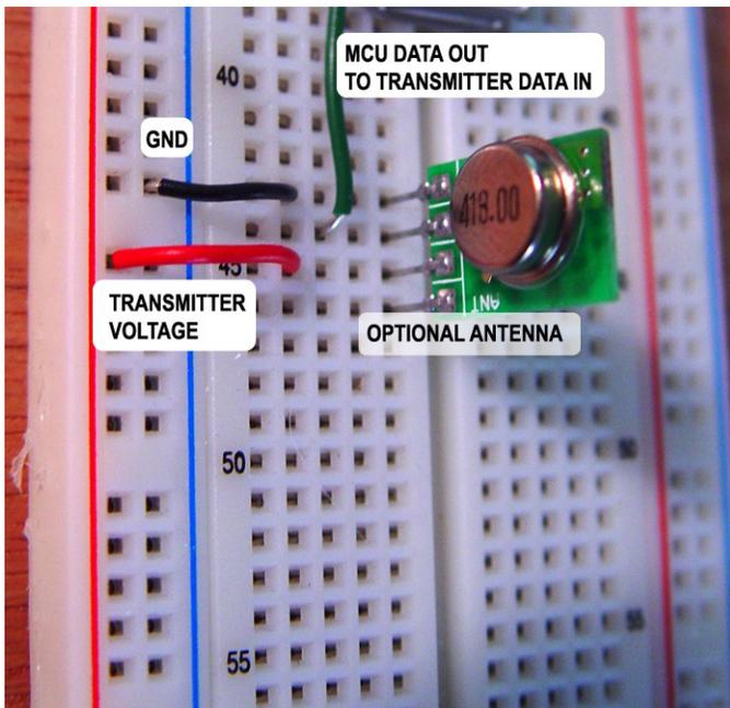
Three of the four transmitter modules have four pins, while the other has six. The six-legged version simply has redundant pins of power and ground, but otherwise remains the same.
