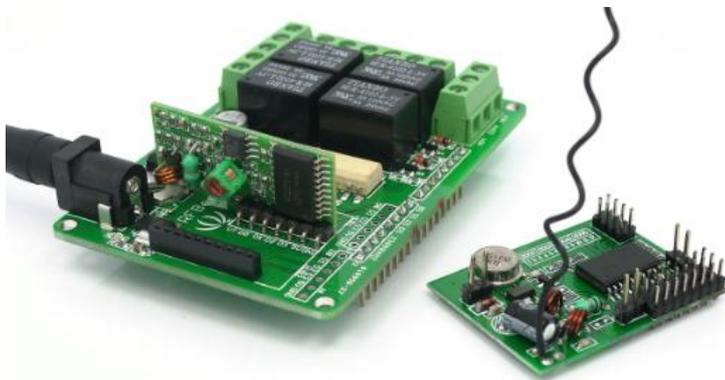
Step1. Plug the Receiver onto the Relay Shield.
