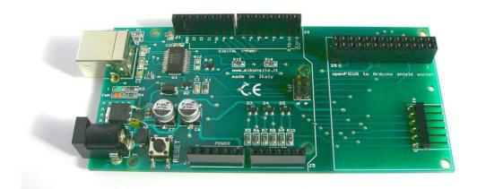
This is a typical Arduino shield
