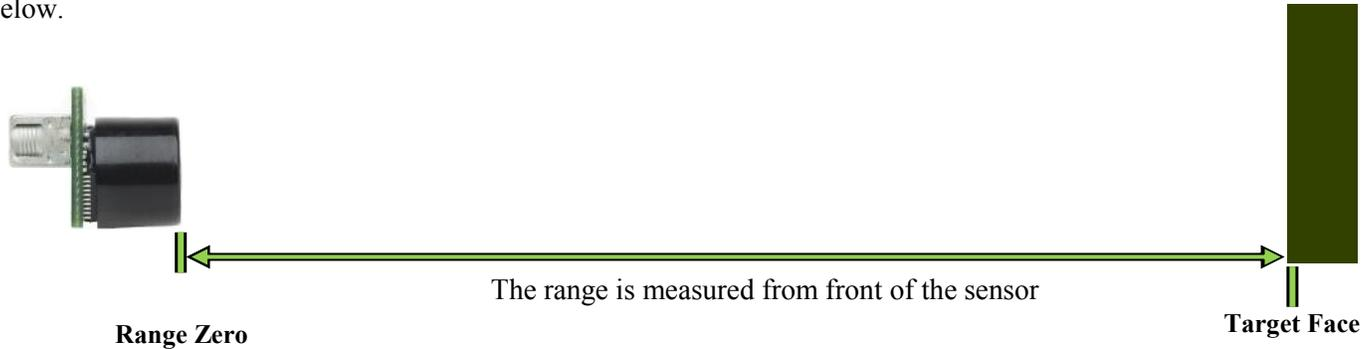
In general, the XL-MaxSonar-EZ will report the range to the leading edge of the closest detectable object. Target detection has been characterized in the sensor beam patterns.
