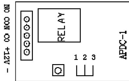
A wireless relay is a codec-adaptive RF receiver with single channel relay. It helps easily deployment of wireless AC control for electrical appliances.
