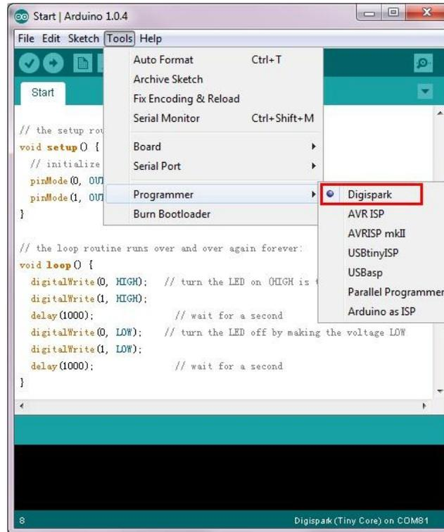
Because there is no reset pin on Tinny85, before pressing the "upload" button to download codes onto Iteaduno Tiny, you need to unplug the USB cable on Iteaduno Tiny first to disconnect the USB connection. Then, press the "upload" button, after 'Plug in device now...' is displayed on IDE window, reconnect the USB cable, and then IDE will download the compiled data onto Iteaduno Tiny. For details about operating procedures, please refer to user manual for Iteaduno Tiny.
