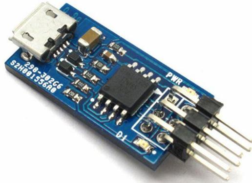
Iteaduino Tiny is a mini development board based on Attiny85 master, which is cheap, compact and easy to use with low power consumption. The mainboard is a derivative board with reference to digispark design, and it supports use of specific Arduino IDE and uses Arduino syntax for programming which is quite convenient.
