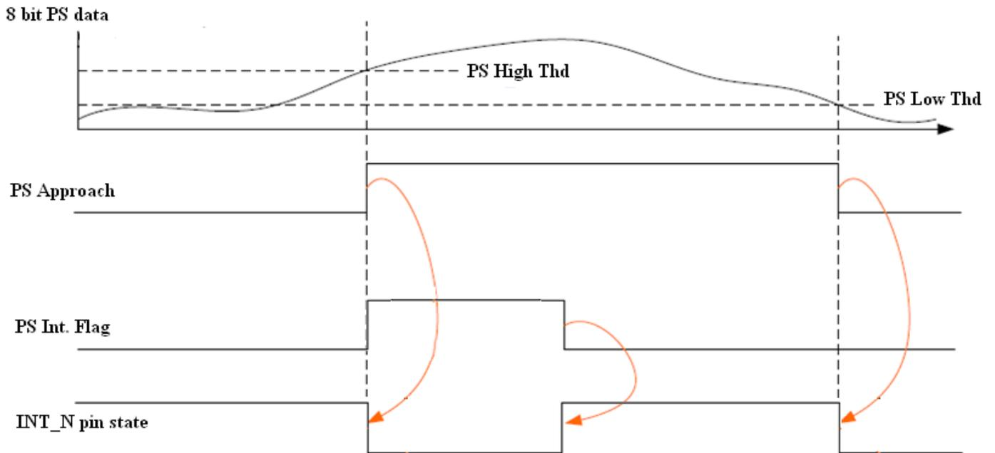
Figure 3. Proximity Sensing Functional Diagram
