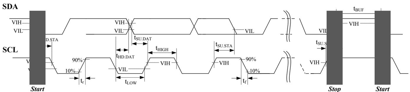
Figure 17. I<sup>2</sup>C Timing Diagram
