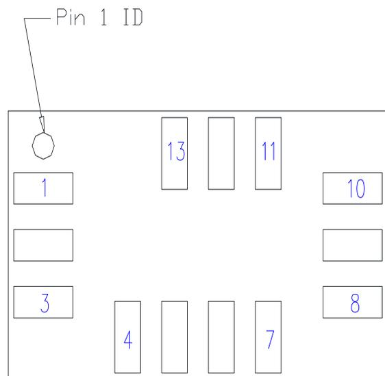
Figure 1. PAJ7620U2 Module Pin Configuration (BTM VIEW)
