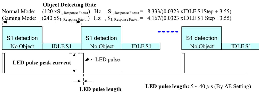
Figure 10. Standby 1 State (S1 state) Diagram
