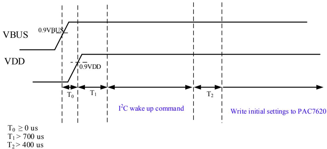
Figure 5. PAJ7620U2 Power-On Timing Diagram
