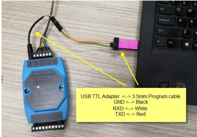
In PC, User needs to set **serial tool**(such as [putty](#), SecureCRT) baud rate to **9600** to access to access serial console for LT. The AT commands are disable by default and need to enter password (default:**123456**) to active it. As shown below:
