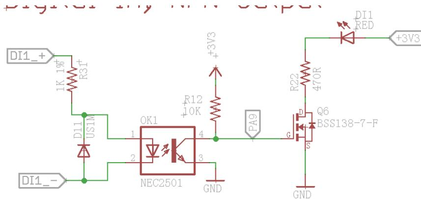
When use need to connect a device to the DI port, both DI1+ and DI1- must be connected.
