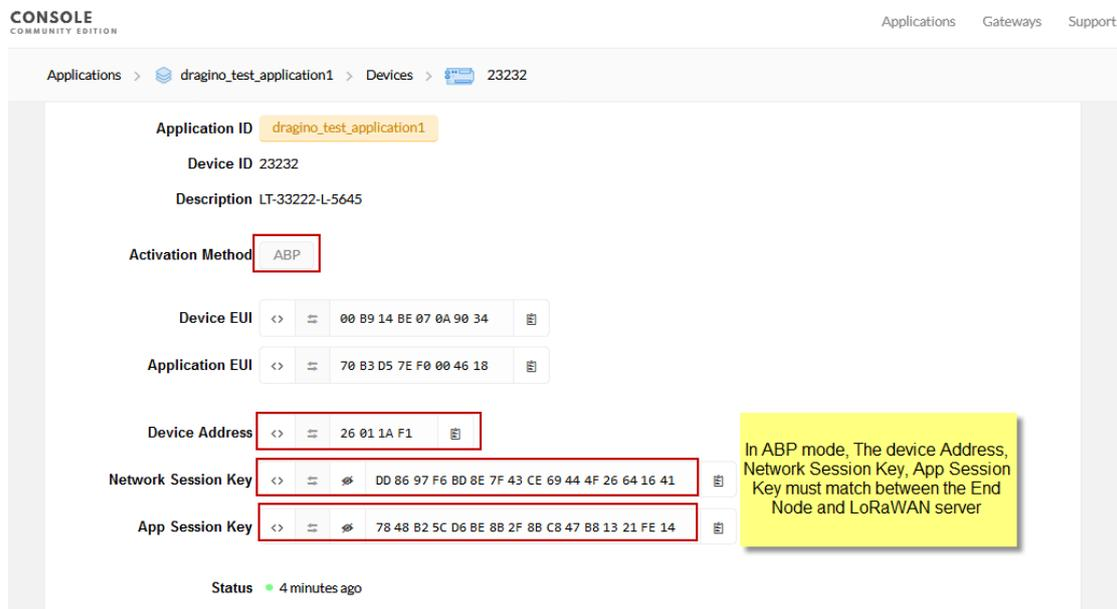
Note: user just need to make sure above three keys match, User can change either in TTN or Device to make them match. In TTN, NETSKEY and APPSKEY can be configured by user in setting page, but Device Addr is generated by TTN.
