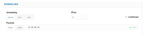
If payload = 0x02010001, while there is load between V+ and DOx, it means set DO1 to low, DO2 to high and DO3 to low. Type code 02 means Digital Output
