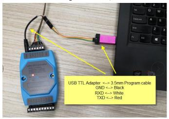
In PC, User needs to set serial tool baud rate to 9600 to access to access serial console for LT. The AT commands are disable by default and need to enter password (default:123456) to active it. As shown below:
