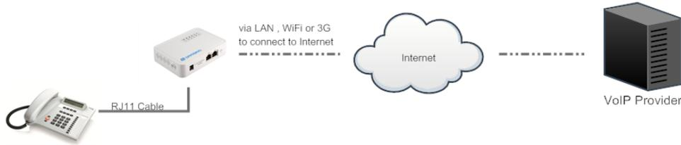
Configure DT01 as a VoIP ATA and make calls via the voip provider
