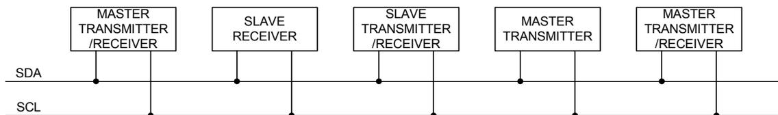
Figure. 5 System configuration
