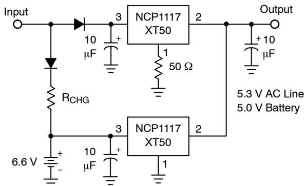
The 50 Ω resistor that is in series with the ground pin of the upper regulator level shifts its output 300 mV higher than the lower regulator. This keeps the lower regulator off until the input source is removed.
