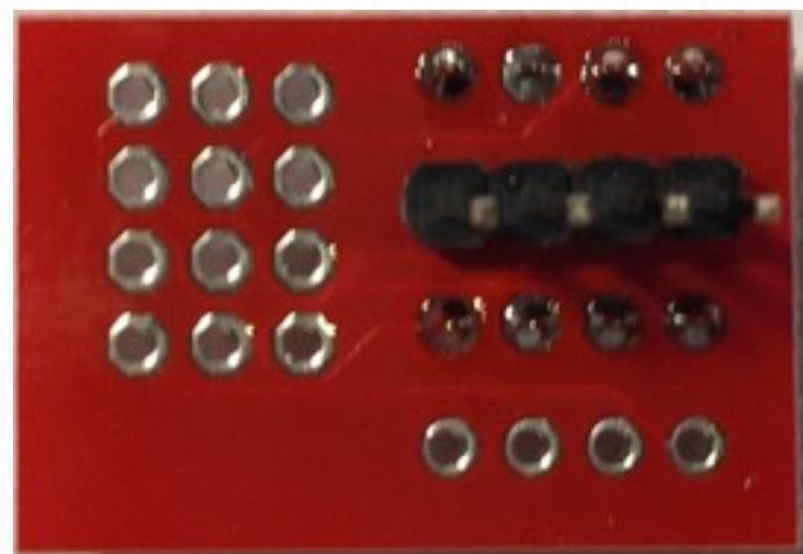
3. Insert the other single row male header strips from the **bottom** of the board into bottom row of holes, and solder it on top.
