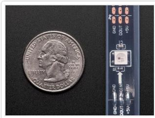
**NeoPixel Digital RGB LED Weatherproof Strip:** 30 LEDs per meter on a black backing strip.
