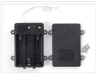
Three alkaline cells (such as AA batteries) can be installed in a [battery holder \(http://adafru.it/771\)](http://adafru.it/771) to provide 4.5 Volts. Though larger and heavier than the fancy lithium-polymer pack, they’re inexpensive and readily available.
