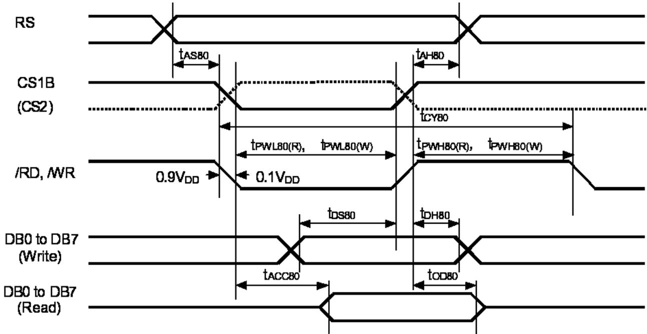
\*\* tPWL80(W) and tPWL80(R) is specified in the overlapped period when CS1B is low (CS2 is high) and /WR(/RD) is low.
