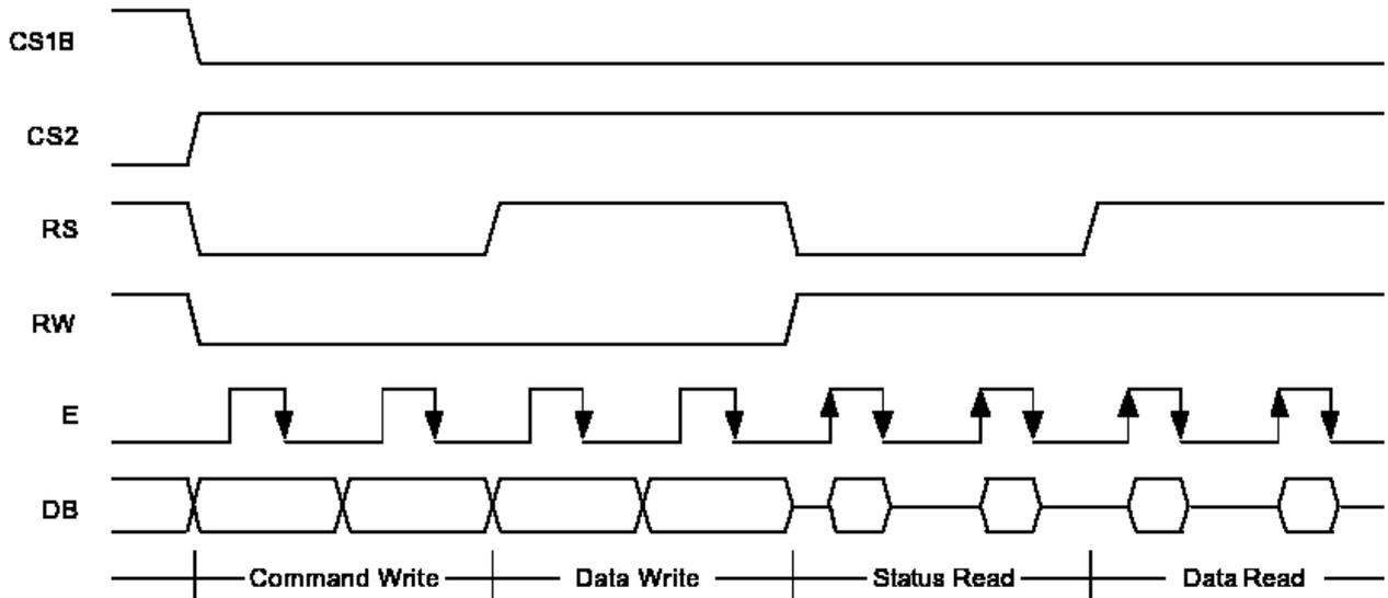
**Figure 1. 6800-Series MPU Interface protocol (PS="H", ME="H")**
