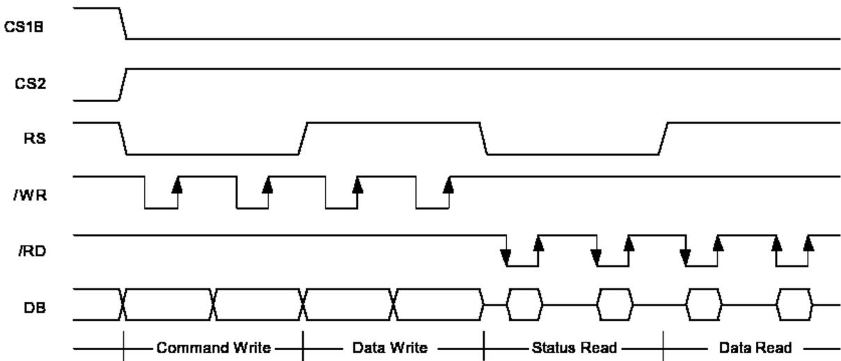
**Figure 2. 8080-Series MPU Interface Protocol (PS="H", ME="L")**
