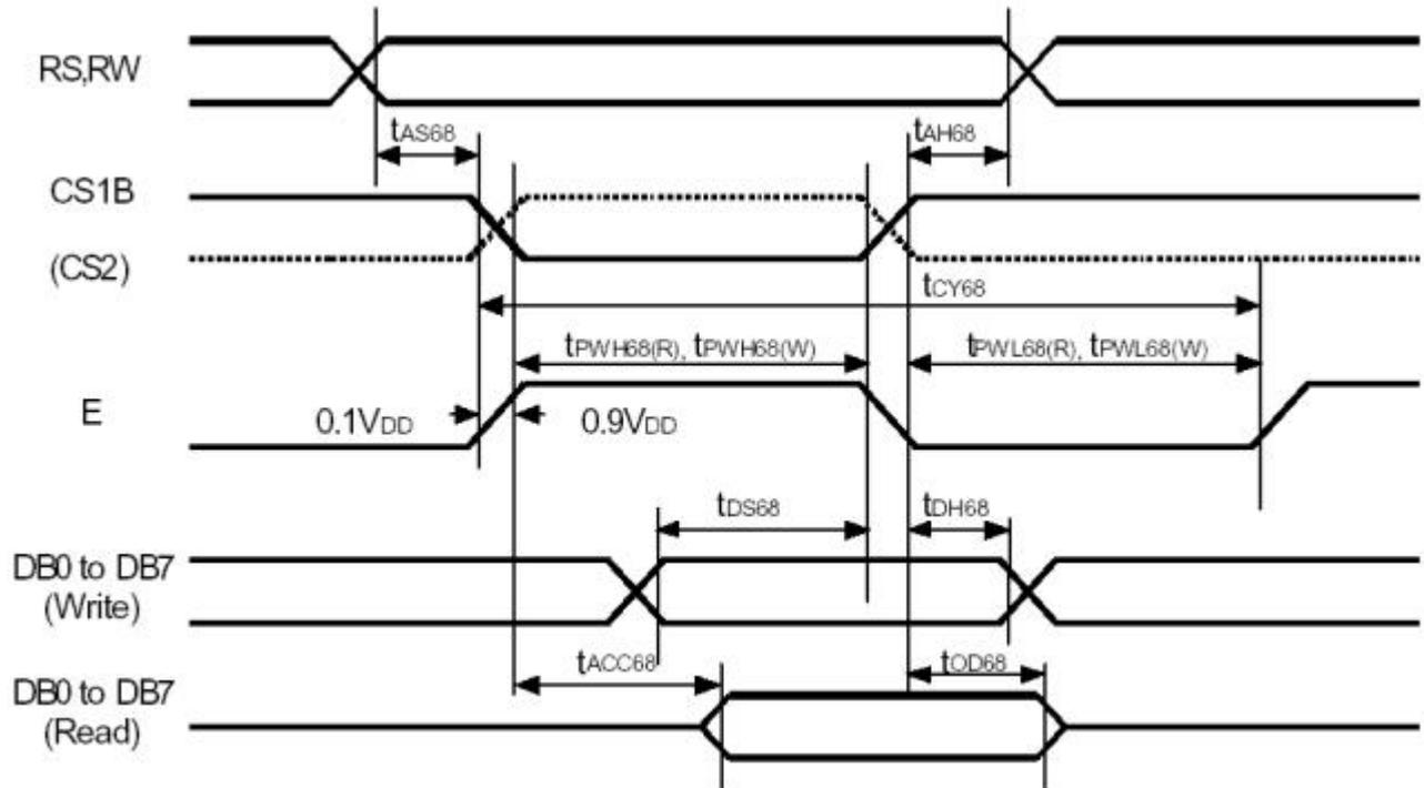
\*\* tPWH68(W) and tPWH68(R) is specified in the overlapped period when CS1B is low (CS2 is high) and E is high.
