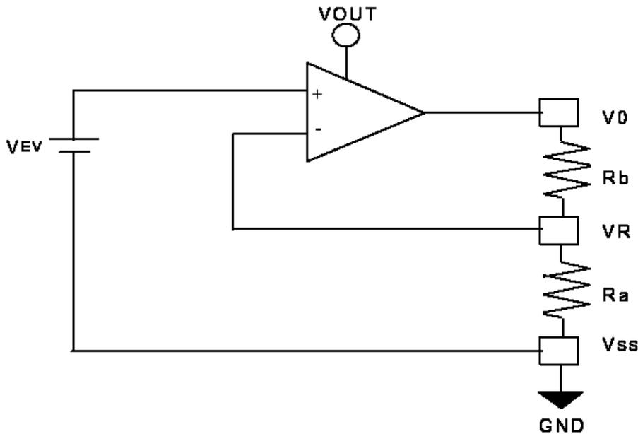
Figure 4. Internal Voltage Regulator Circuit
